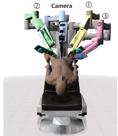
4-Arm da Vinci System (set-up assumes left-side assistant)
